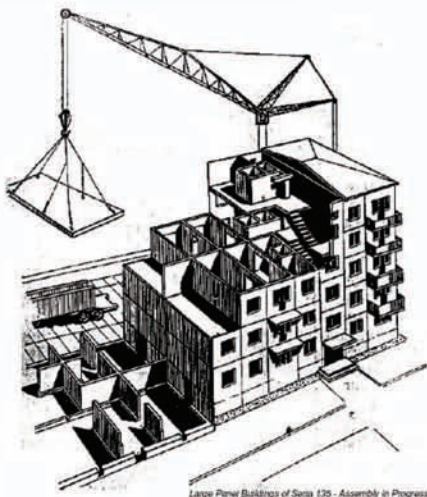
Large Panel Buildings of Sana 135 - Assembly in Progress
